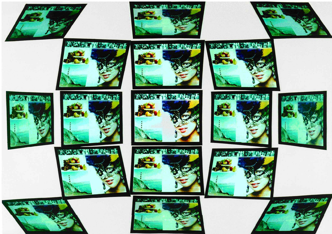
Figure 9. Photographs of a 4-domain CTN TFT panel. Viewing angles are 0° (centre), 30° (middle) and 50° (outer); azimuthal angles are at 45° intervals.
